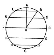
upon a wharf wall, as at A in the annexed diagram, and also the point of lowest depression as at G, and a circle drawn through these two extreme points, then, roughly, the heights at equal successive times may be found by dividing the circumference of the circle into equal parts, as at B, C, D, &c., the fall and succeeding rise of the water reaching the points thus found in equal times. If now, for sim-
